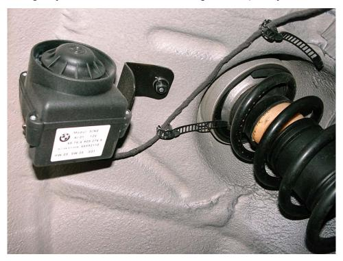
If the alarm is triggered, the emergency siren issues an acoustic signal. A short acoustic signal is also triggered when locking/unlocking.
